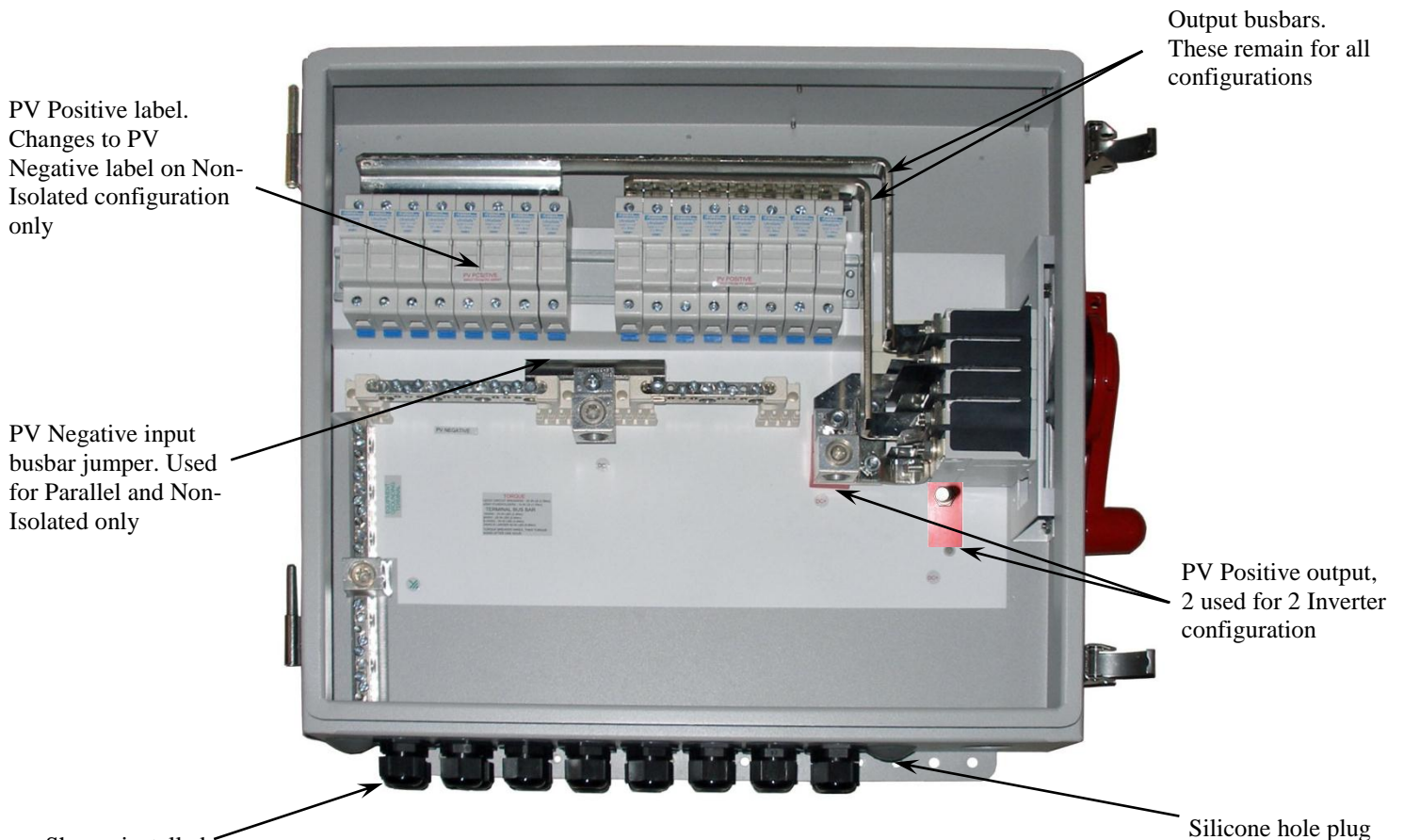
MNPV16HV Parallel configuration (default). 16 string Disconnecting Combiner
