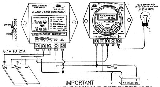
PANEL ISOLATION DIODES ARE USUALLY INSTALLED BY THE SOLAR PANEL MANUFACTURER TO PREVENT FLOW OF ELECTRICITY FROM ILLUMINATED PANELS INTO SHADED PANELS. SIMPLY CONNECT THE CHARGE INDICATOR WIRE TO THE ANODE SIDE OF THE BLOCKING DIODE ON ANY ONE OF THE PANELS.
