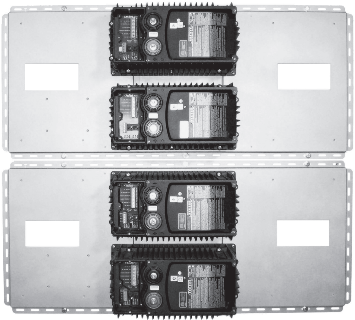
Figure 5: Four FXs installed on FW-MPs
